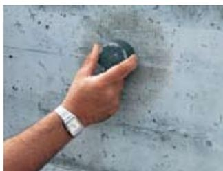
Smoothen test area with a grinding stone.
